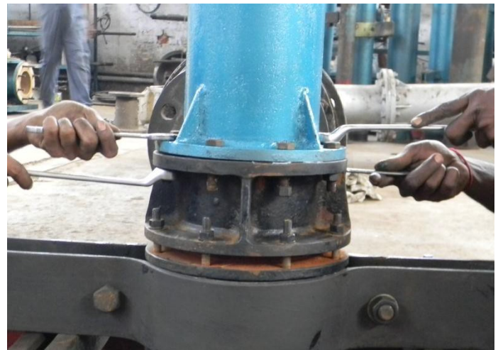
Figure 13 – Tightening the fasteners in diametrical fashion in the assembly
