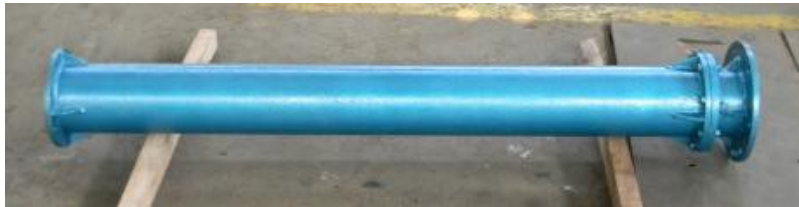
Figure 8 – Resting Column Pipe on Wooden Planks
