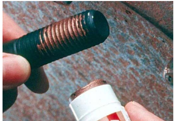
Figure 6 – Applying Anti-Seize Paste on the Threaded end of Impeller Shaft
