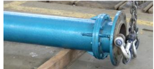
Figure 9 – Mounting Eye-bolts, chain & shackles on Top Flange face
