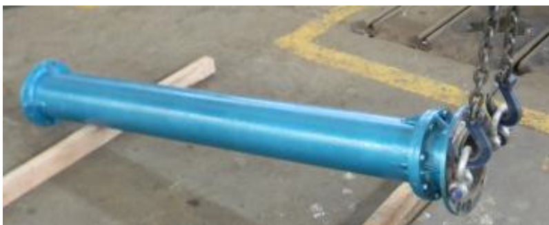
Figure 10 – Lifting the Column Pipe
