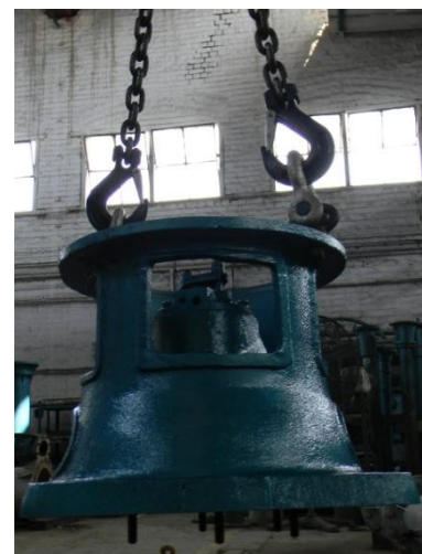
Figure 25 – Lifting the Discharge Head
