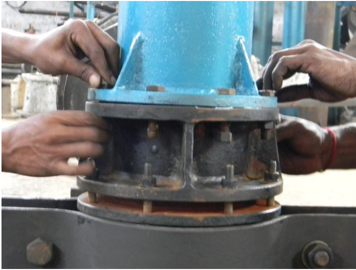
Figure 12 – Assembling the Column Pipe with Bowl Assembly
