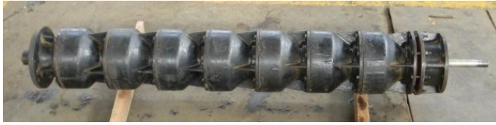
Figure 2 – Resting the Bowl Assembly
