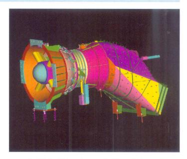
☐ 6 X 16000 kW and 2 X 22000 kW Volute Pump Turbines under execution.
