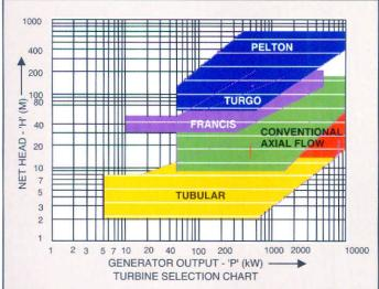
NOTE: Approx. discharge requirement can be worked out using equation, Q = K x P/H Cumec, where K=0.12 to 0.13
